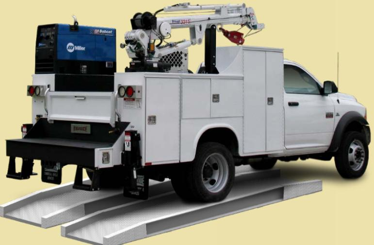
**The Mark-I temporary crossing platforms are designed for utility and emergency vehicle access. Engineered with structural, marine grade metals, they offer high strength and durability in a light and nimble form factor for rapid deployment and minimal support equipment.**
